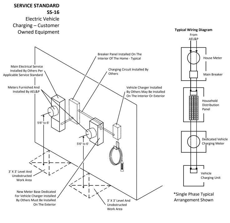
Service Equipment, Circuits, Meter Bases, Chargers And Conduit To Be Installed By Customer.
