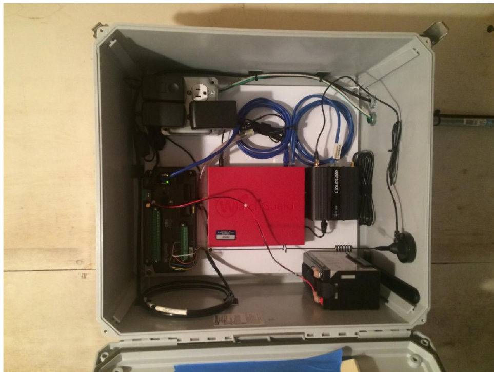
Figure 3. Showing the streamgage data logger and transmitter.
